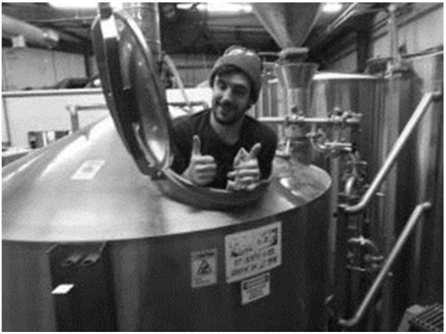
What's wrong inn this picture? Asphyxiation is the leading cause of death in confined spaces. A permit-required confined space may contain a hazardous atmosphere due to the displacement of oxygen by grape fermentation byproducts during the fermentation process, when sugar is converted into water, alcohol and carbon dioxide.
