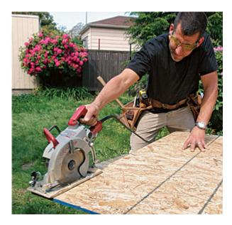
**Prevention strategy:** Keep the blade sharp, use the saw at the speed the manufacturer recommends and properly support the stock being cut—remember, using your legs is not a proper means of support!
